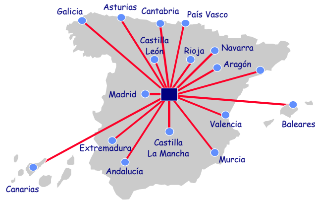
Figure 1. Topology of the RedIris IP/ATM backbone
